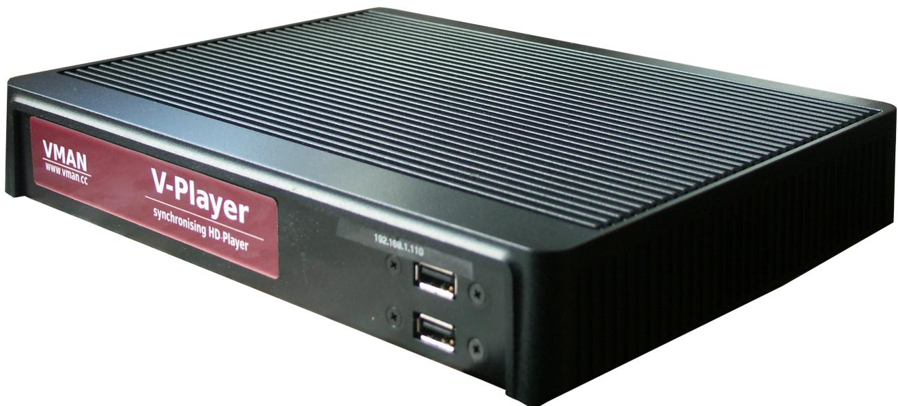
V-Player comes with an integrated software EDID manager. If V-Player is connected to a device without EDID (e.g. matrix switch, LED processor, projector or fiber transmitter), an internal EDID can be used with no need to connect an external hardware EDID manager / detective.
